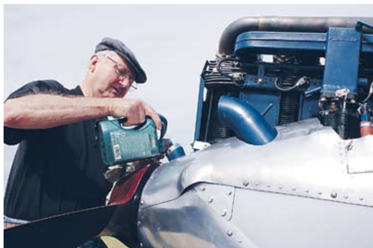
Left: Bob McGarry tops up the oil, a wet sump system on the upright Gipsy engine.
